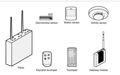
Figure 1: System components
